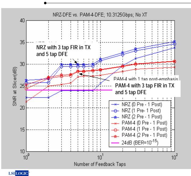
•Transmit equalization is a FIR with one tap to address postcursor ISI and varying number of taps to address pre-cursor ISI.
