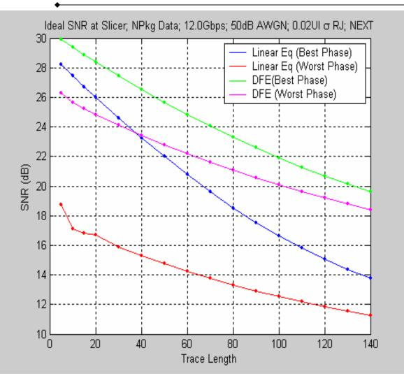
•The benefit of DFE is shown to grow with the amount of high frequency noise and the amount of high frequency boost required to compensate for the channel's attenuation.
