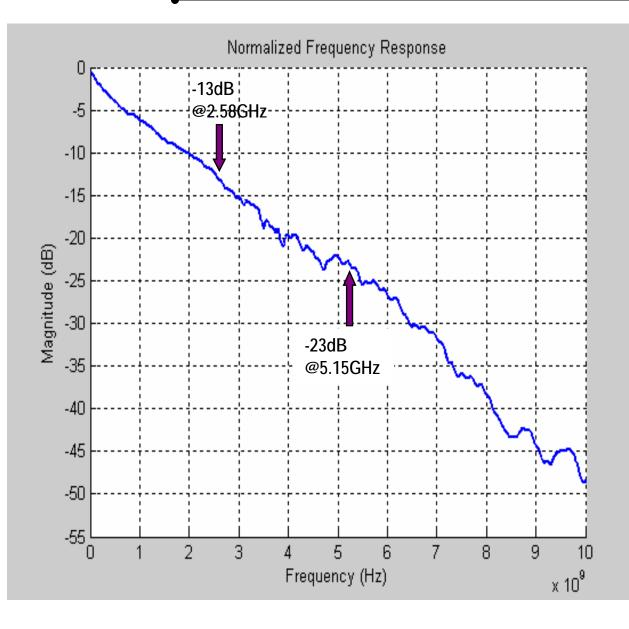
•Difference between response at 5.15GHz (Nyquist frequency of NRZ) and 2.58GHz (Nyquist frequency of PAM-4) is about 10dB.
