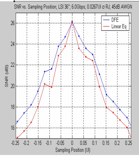
•Even without crosstalk, the benefit of DFE can be seen as the sampling position moves away from the center of the eye. This results in improved jitter tolerance.
