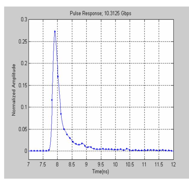
•Pulse response generated assuming single pole TX lowpass filter with corner at <sup>3</sup>/<sub>4</sub> \* baud rate.
