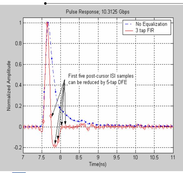
•Transmit equalization is three tap FIR with one tap to address pre-cursor ISI and one tap to address post-cursor ISI. (One tap post-emphasis and one tap pre-emphasis.)
