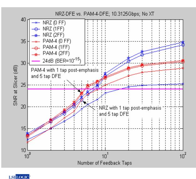
•Transmit equalization is FIR with varying number of taps to address pre-cursor ISI.
