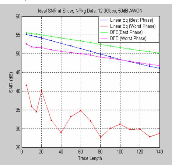
•DFE has an advantage over linear equalizer at the ideal sampling phase because it results in less noise enhancement.
