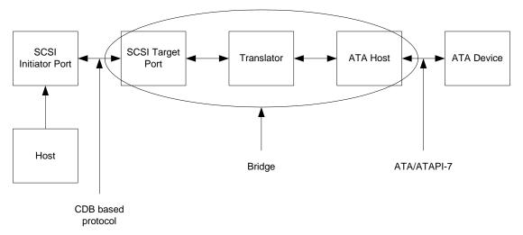
The bridge is composed of a SCSI Target, an ATA Host, and a translator. The translator receives CDB's from the SCSI Target, converts them to ATA/ATAPI-7 commands, and issues them to the ATA device using the ATA Host. The SCSI Target may be conceptual, possibly only existing in software; or it could be any device that receives SCSI CDB's including a SAS Target, 1394 device, USB, etc. The ATA Host shall be one of the following:
