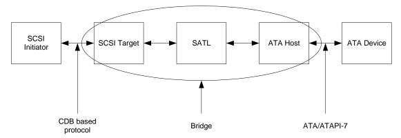
The bridge is composed of a SCSI Target, an ATA Host, and a SCSI to ATA Translation Layer (SATL). The translator receives CDB's, converts them to ATA/ATAPI-7 commands, and issues them to the device using the ATA Host. The SCSI Target may conceptual, possibly only existing in software. The ATA Host shall be a standard SATA or PATA ATA/ATAPI-7 compliant host.
