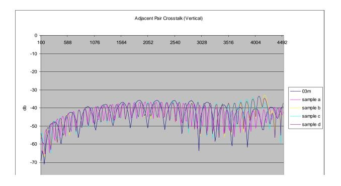
Even pair crosstalk is between RX0/RX1, TX0/TX1, RX2/RX3, TX2/TX3. The results are similar for odd pairs.
