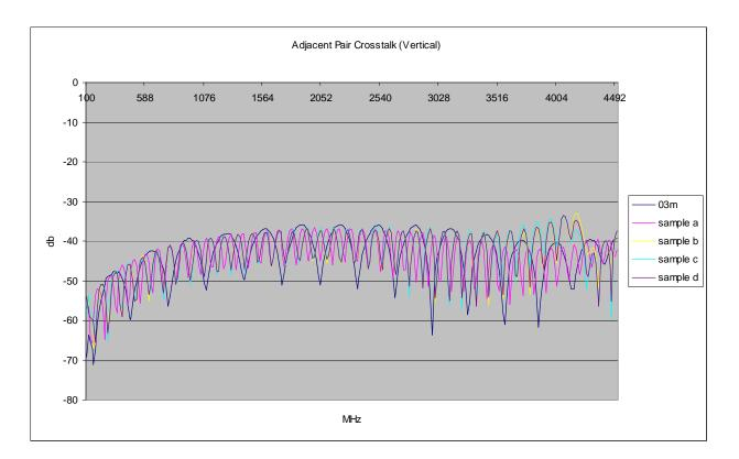
Even pair crosstalk is between RX0/RX1, TX0/TX1, RX2/RX3, TX2/TX3. The results are similar for odd pairs.
