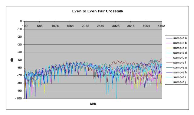
End-to-end crosstalk is between any pair of the group RX0, TX0, RX1, TX1 to any pair of the group RX2, TX2, RX3, TX3. In this case, the crosstalk spans the section of the connector reserved for sidebands.
