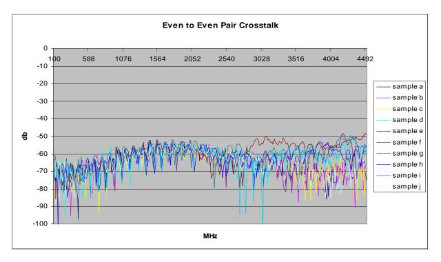
End-to-end crosstalk is between any pair of the group RX0, TX0, RX1, TX1 to any pair of the group RX2, TX2, RX3, TX3. In this case, the crosstalk spans the section of the connector reserved for sidebands.
