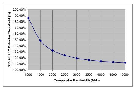
As can be seen, in order to minimize the frequency-dependent effects, the comparator bandwidth must be maximized, and in fact even with a bandwidth of 4,5 GHz there is still an amplitude error of 13%. In practice, additional second order effects (not modeled in these simulations) tend to accumulate, increasing the frequency-dependent amplitude error even more.
