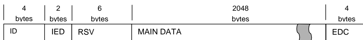
Figure 2 – Logical Layout of a DVD+RW Data Sector
