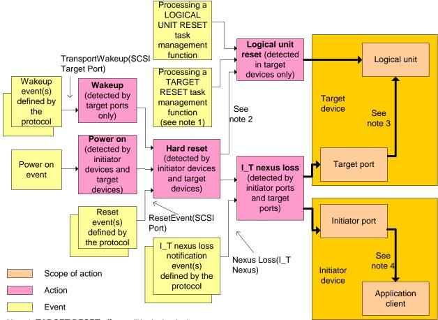
Note 1: TARGET RESET affects all logical units in a target device to which the I\_T nexus has access.
