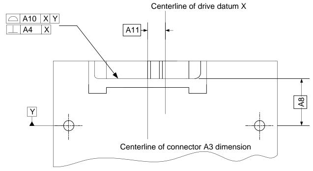
Figure 5-1 2.5" DRIVE FORM FACTOR WITH SAS CONNECTOR
