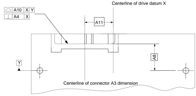
Figure 5-1 3.5" DRIVE FORM FACTOR WITH SAS CONNECTOR
