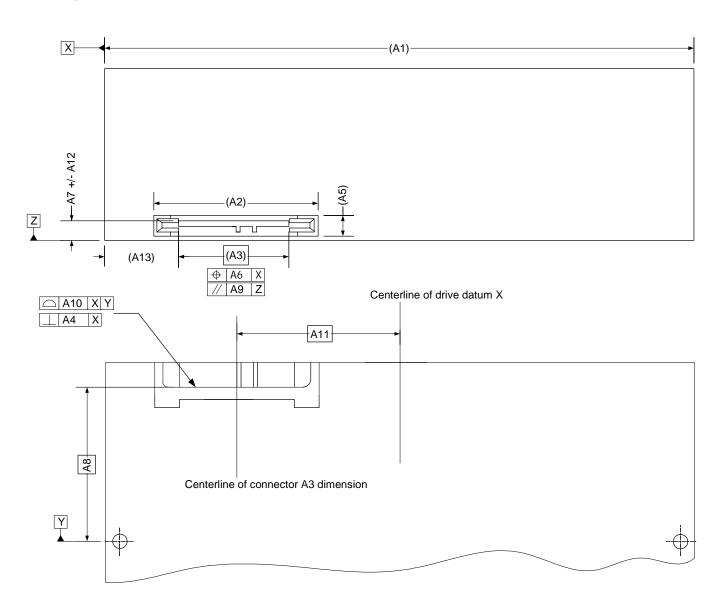
Figure 5-1 5.25" DRIVE FORM FACTOR WITH SAS CONNECTOR
