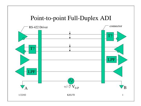
A low impedance line termination is optional if the distance and driver output transition times are bounded.
