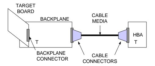
TERMINATORS, T, ARE ATTACHED TO THE BACKPLANE AND HBA BOARDS
