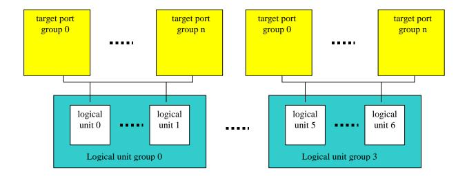
For example, virtual logical units formed from one physical logical unit (e.g. virtual disk drive volumes created from the same physical disk) may need to share the same target behavior port asymmetric access states.
