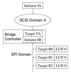
SCSI Domain A uses a non-interlocked protocol such as FCP or FCP-2. Targets B0, B1, etc. are normal parallel SCSI disk drives. The bridge controller is a parallel SCSI to Fibre Channel adapter (JBOD), presenting the devices behind it as individual LUNs. For example, it might present target B0 LUN 0 as its LUN 0, target B1 LUN 0 as its LUN 1, etc.
