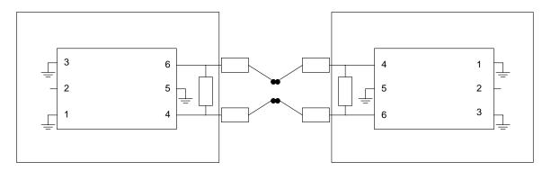
Using a network analyzer, measure the insertion loss (S<sub>21</sub>) of the joined test fixtures. Store this measurement into network analyzer memory. Detach to fixtures from each other, install sample. Set the network analyzer to display {S<sub>21</sub>  $\div$  Memory}, which is the insertion loss of the cable with the fixture contribution removed. Set IF BW to  $\leq$  100 Hz to eliminate spurious data.
