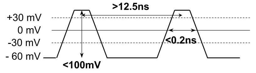
Positive going differential pulse train based at -60 mV
