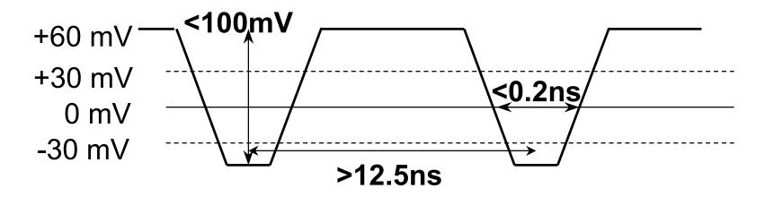
Negative going differential pulse train based at +60 mV
