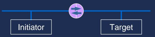
SBP-2 relies upon bus reset to synchronize state between controller and target
