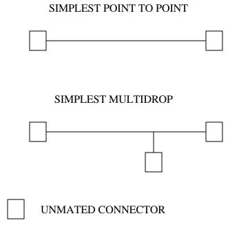
The point to point construction allows inclusion of connectors and transition regions, multiple line cross talk, resonance issues and other issues not previously considered in uniform cable media.
