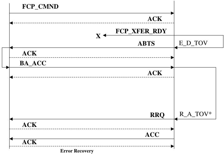
For Class 2 the BA\_ACC indicates that the FCP\_XFER\_RDY was never received by the Initiator. (BA\_ACC Payload is SEQ\_ID invalid, low SEQ\_CNT=0, high SEQ\_CNT =SEQ\_CNT in ABTS frame = 1.) Both Target and Initiator must establish Recovery Qualifiers. The value for R\_A\_TOV\* for in-order delivery is 0. A new SEQ\_ID must be used in the retransmission of FCP\_XFER\_RDY. The use of REC to determine status for error recovery is optional.
