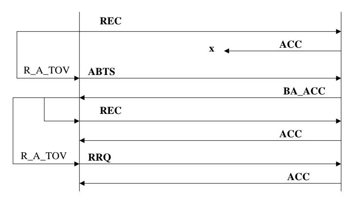
Since the Target has already responded with ACC then no context exists for the Exchange. The Target would view the ABTS as being issued on a new Exchange, establish a Recovery Qualifier and respond with BA\_ACC (Payload is SEQ\_ID invalid, low SEQ\_CNT=high SEQ\_CNT= SEQ\_CNT of ABTS). Since REC does not change any state, it can be reissued unconditionally. The second REC must be issued in a new Exchange.
