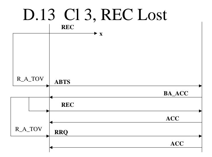
Since the REC was never received by the Target, the BA\_ACC payload is SEQ\_ID invalid, low SEQ\_CNT =0, high SEQ\_CNT= SEQ\_CNT of ABTS=1. Recovery qualifiers are established on both sides The second REC must be issued in a new Exchange
