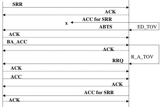
Note: The BA\_ACC payload indicates SEQ\_ID invalid, low SEQ\_CNT=0 and high SEQ\_CNT=SEQ\_CNT of the ABTS, which indicates that the ACC for SRR was not received and will be discarded if it is received. Recovery Qualifiers are established on both sides. The ACC for SRR is issued with a new SEQ\_ID.
