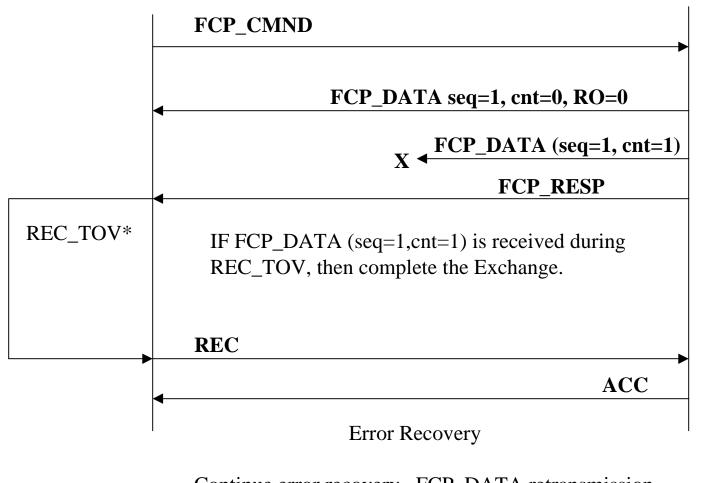
Continue error recovery. FCP\_DATA retransmission must use a new SEQ\_ID. For in-order delivery, the value of REC\_TOV\* is 0.
