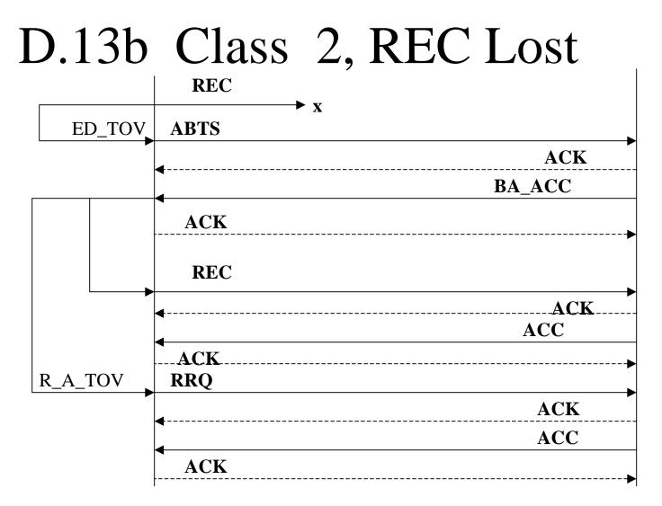
The BA\_ACC payload indicates that the REC was never received by the Target (Payload is SEQ\_ID invalid, low SEQ\_CNT=0, high SEQ\_CNT= SEQ\_CNT in ABTS frame) Recovery Qualifiers are established on each side.
