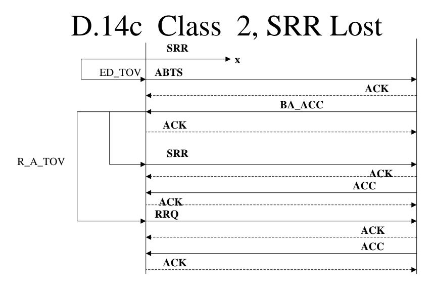
Since this is an ABTS on a new Exchange, Recovery Qualifiers must be established. BA-ACC indicates Invalid SEQ\_ID, low SEQ\_CNT= 0 and high SEQ\_CNT = SEQ\_CNT of the ABTS. The second SRR is issued using a new Exchange.
