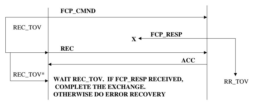
For Sequence level recovery, the Target must keep the context of this Exchange until the OX\_ID value is reused in a new command, implicitly validating the receipt of FCP\_RESP, or for at least RR\_TOV, in order to preserve the FCP\_RESP information. This long timeout can be avoided by using FCP\_CONF. The FCP\_RESP retransmission must use a new SEQ\_ID.
