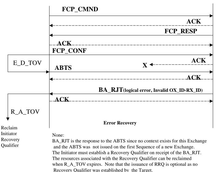
D.5? Class 2 Multiple Error Condition, Abort the Exchange
