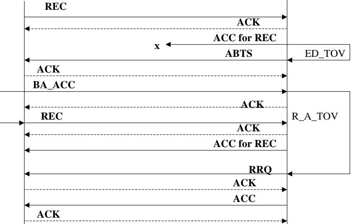
Note: The Target determines that the ACC was never received by the Initiator; BA\_ACC payload is SEQ\_ID invalid, Low SEQ\_CNT=0, High SEQ\_CONT= SEQ\_CNT of ABTS. After responding to the ABTS, the Initiator reissues the REC in a new Exchange.
