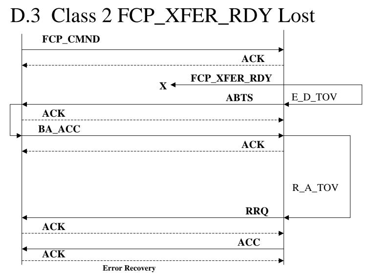
For Class 2 the BA\_ACC indicates that the FCP\_XFER\_RDY was never received by the Initiator. (BA\_ACC Payload is SEQ\_ID invalid, low SEQ\_CNT=0, high SEQ\_CNT =SEQ\_CNT in ABTS frame = 1.) Both Target and Initiator must establish Recovery Qualifiers. A new SEQ\_ID must be used in the retransmission of FCP\_XFER\_RDY. The use of REC to determine status for error recovery is optional.
