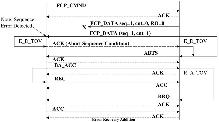
BA\_ACC indicates by its payload, that the FCP\_DATA Sequence was not completely received(Payload: SEQ\_ID invalid, low SEQ\_CNT of 0 not equal to high SEQ\_CNT of the ABTS frame of 2). A new Sequence ID shall be used for retransmission of FCP\_DATA. Note that if all data frames arrive at the initiator before E\_D\_TOV expires, then no recovery is required; a frame or frames arrived out-of-order. The ACKs for REC/ACC are not shown.
