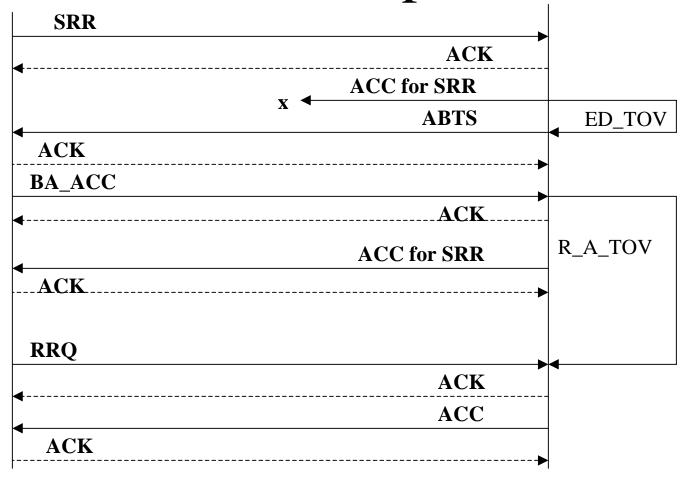
Note: The BA\_ACC payload indicates SEQ\_ID invalid, low SEQ\_CNT=0 and high SEQ\_CNT=SEQ\_CNT of the ABTS, which indicates that the ACC for SRR was not received and will be discarded if it is received. The ACC for SRR is issued with a new SEQ\_ID and a SEQ\_CNT one greater than used in the ABTS.
