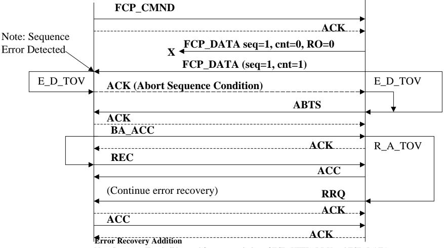
New Sequence IDs shall be used for retransmission of FCP\_XFER\_RDY and FCP\_DATA. For Class 2, the Sequence count value used with the retransmission of FCP\_DATA shall be one greater than the value used in ABTS. Note that if all data frames arrive at the initiator before E\_D\_TOV expires, then no recovery is required; a frame or frames arrived out-of-order. The ACKs for REC/ACC are not shown.
