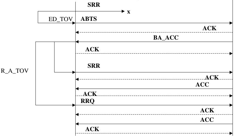
Note: The second SRR is issued using a new Exchange. Since this is an ABTS on a new Exchange, a Recovery Qualifier must be established by the Target. BA-ACC indicates Invalid SEQ\_ID, low SEQ\_CNT= 0 and high SEQ\_CNT = SEQ\_CNT of the ABTS.
