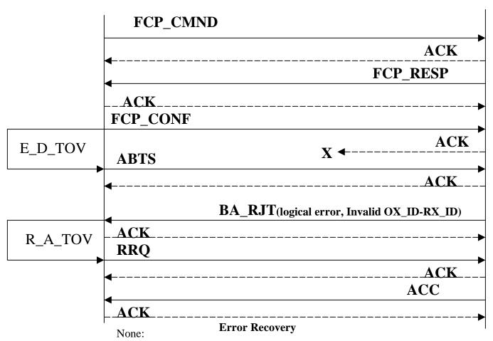
The Initiator must establish a Recovery Qualifier on receipt of the BA\_RJT. The resources associated with the Recovery Qualifier can be retired on the receipt of the ACK (out of order) or when R\_A\_TOV Time-out has expired. Note that the issuance of RRQ is optional as no Recovery Qualifier was established by the Target.
