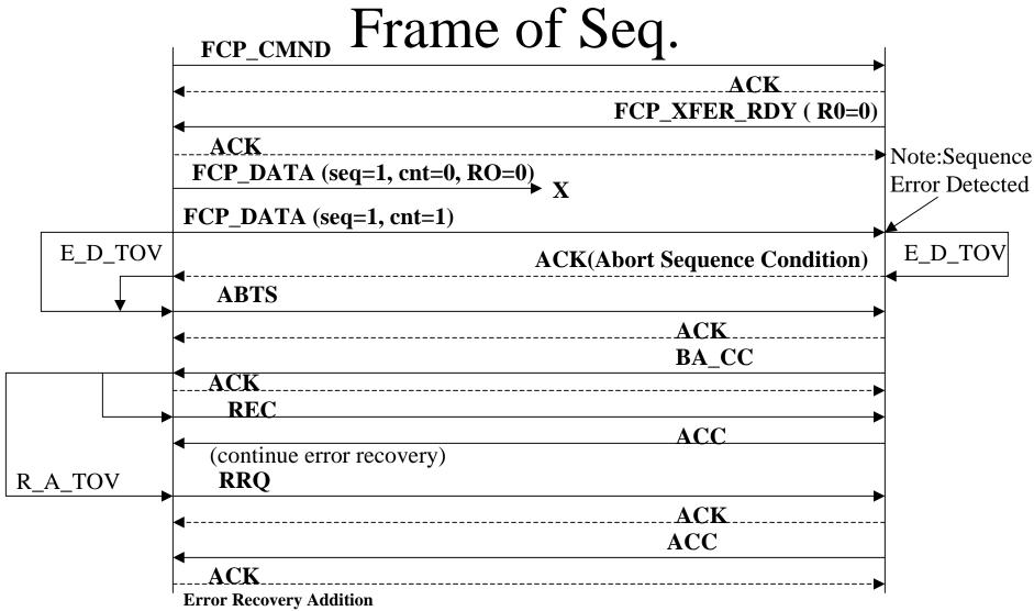
New Sequence IDs shall be used for retransmission of FCP\_XFER\_RDY and FCP\_DATA. For Class 2, the Sequence count value used with the retransmission of FCP\_DATA shall be one greater than the value used in ABTS. Note that if all data frames arrive at the Target prior to the expiration of E\_D\_TOV,( out-of-order) then then is no error and no recovery is necessary. ACKs for REC/ACC are not shown.
