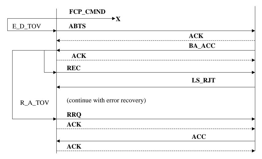
Note: BA-ACC payload: SEQ\_ID Validity = invalid, Low SEQ\_CNT= 0, High SEQ\_CNT = SEQ\_CNT of ABTS frame. The ACKs for REC/LS\_RJT are not shown.
