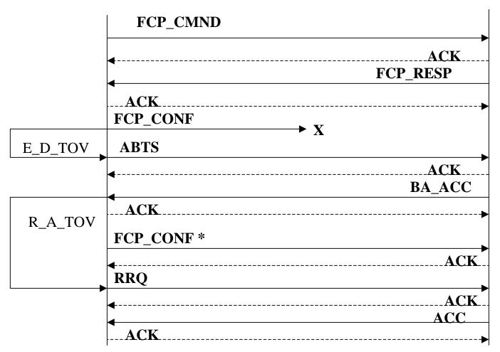
BA\_ACC payload indicates that FCP\_CONF was not received (Low SEQ\_CNT not equal to High SEQ\_CNT value of the ABTS)
