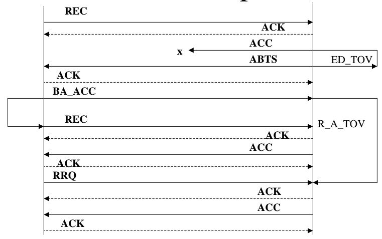
Note: The second REC is issued using a new Exchange. Since REC does not change any state, it can be reissued unconditionally.
