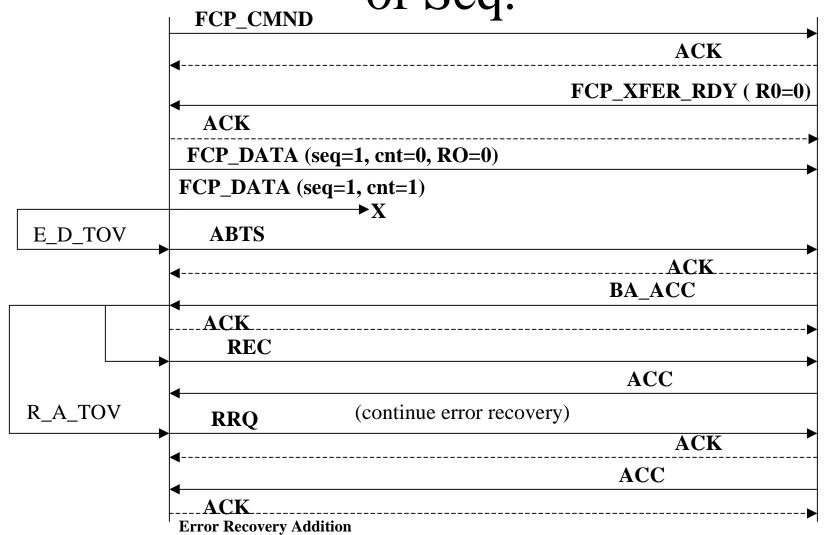
New Sequence Ids shall be used for the retransmission of FCP\_XFER\_RDY and FCP\_DATA. For Class 2, the starting Sequence count value used with the retransmission of FCP\_DATA frames shall be one greater than the value used in ABTS. The ACKs for REC/ACC are not shown.
