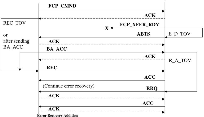
A new SEQ\_ID must be used in the retransmission of FCP\_XFER\_RDY. For Class 2, the SEQ\_CNT value used must be one greater than the value used in the ABTS frame. The ACKs for REC/ ACC are not shown.
