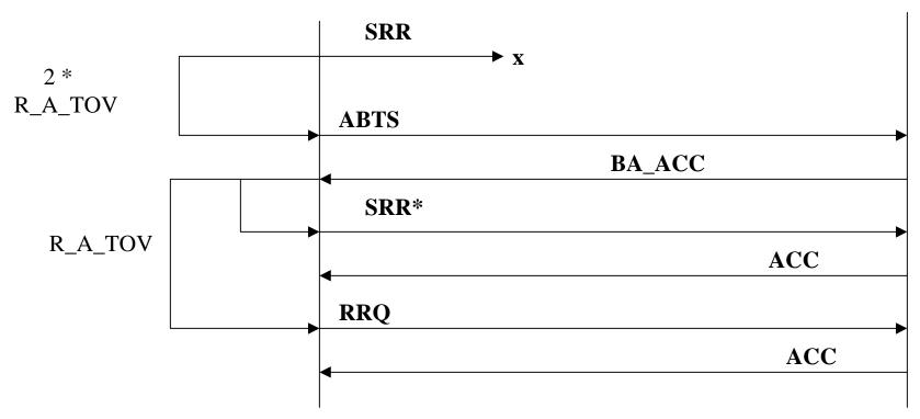
Note: BA\_ACC Payload: SEQ\_ID Validity = invalid, Low SEQ\_CNT=x'0000', High SEQ\_CNT = SEQ\_CNT of ABTS. SRR\* is issued in a new Exchange. The Target restarts the original Exchange per the SRR\* Payload.
